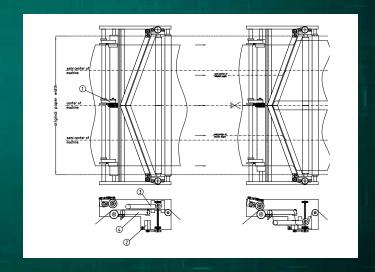
The unit can be fully controlled from the machine room, either as a stand-alone unit or even fully integrated into the press controls. The flexweb has no influence on the register stability or running speed of the machine and even webbing up can be done as normal.
